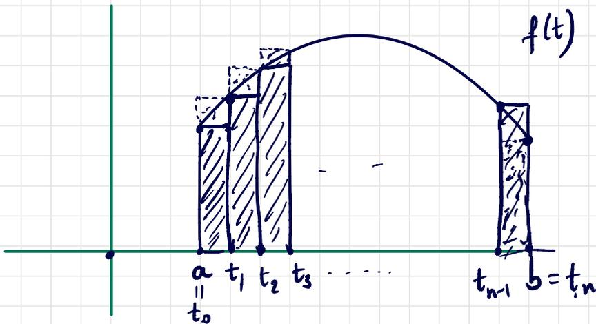
We divide the interval  $[a, b]$  into  $n$  equal subdivisions each of width  $\Delta t = \frac{b-a}{n}$  ← length of  $[a, b]$
